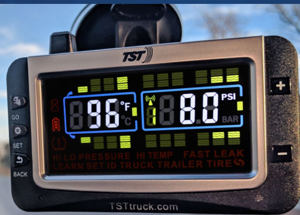
TST WIDE-SCREEN COLOR DISPLAY Real-time alerts for Tire Pressure and Temperature
